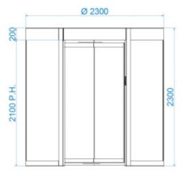
Concrete Base to specification at least (cube) 30N/mm2 of resistance. Base to be flat and level to  $\pm -5mm$  over footprint area. Dimensions to be  $\pm 2250 \times 2250 \times 150$  deep min. (units in mm).
